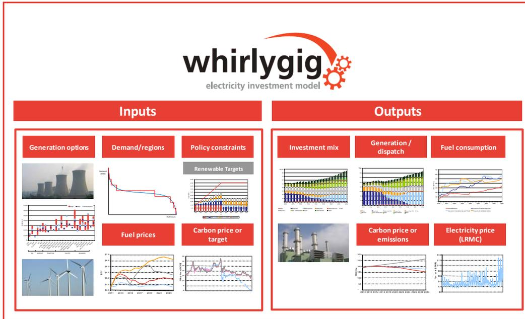
For the stand-alone LRMC, *WHIRLYGIG* has been used to model each load shape for each year *independently*. That is, for a given load shape *WHIRLYGIG* has not been used to determine an optimal investment path over the four years of the modelling period but rather an optimal investment mix for each year independently.
